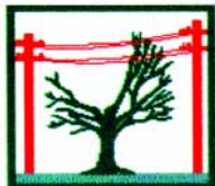
Fig 1. Example of top direct trimming done to trees with a decurrent growth habit.
